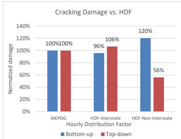
Figure A.3. Effect of hourly distribution factor (HDF) on predicted fatigue damage
