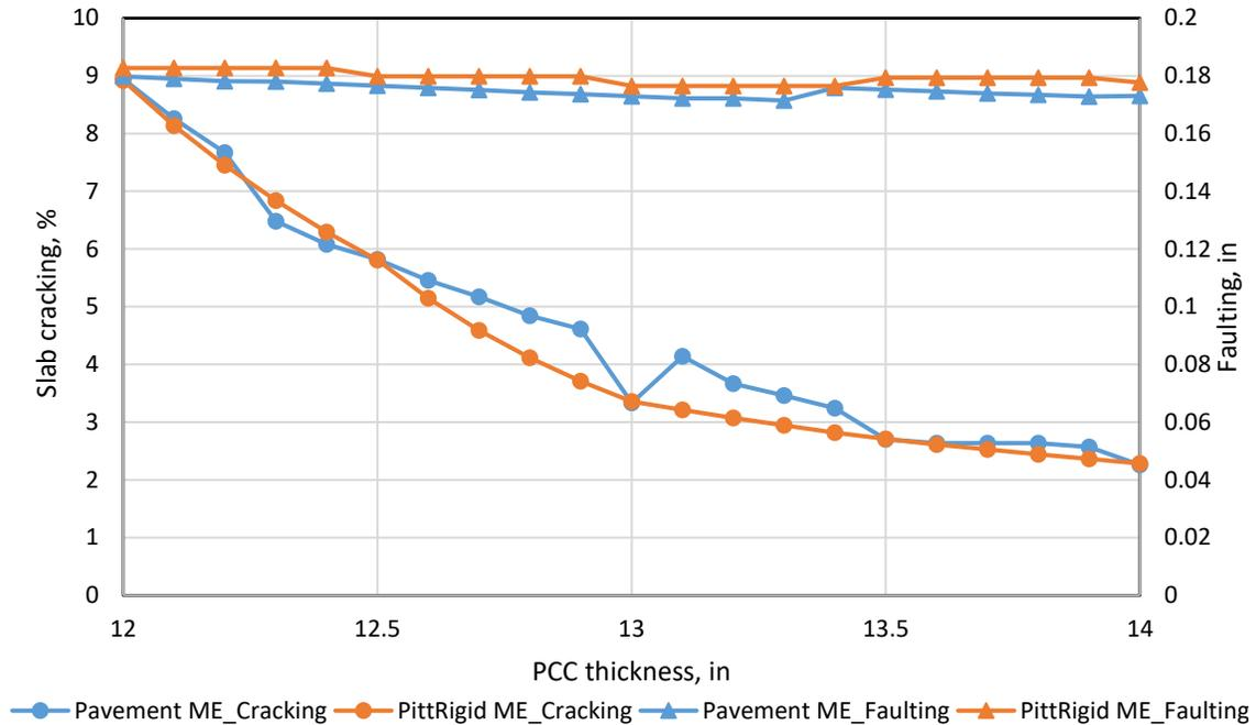
Figure 4-12. Comparing slab cracking and faulting predictions between Pavement ME and PittRigid ME at 90% reliability with respect to PCC thickness for Case 5
