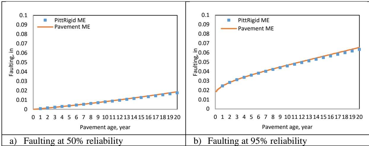
Figure 4-7. PittRigid ME and Pavement ME joint faulting prediction comparisons for Case 1
