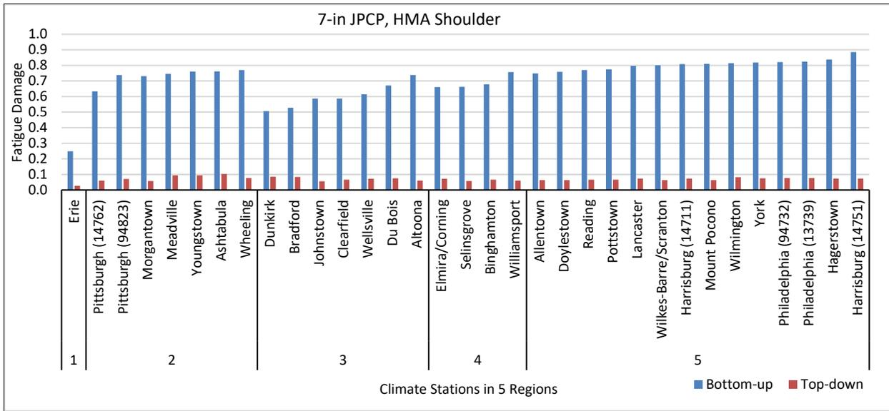
Figure A.7. Predicted fatigue damage for all climate stations, a 7-in thick JPCP
