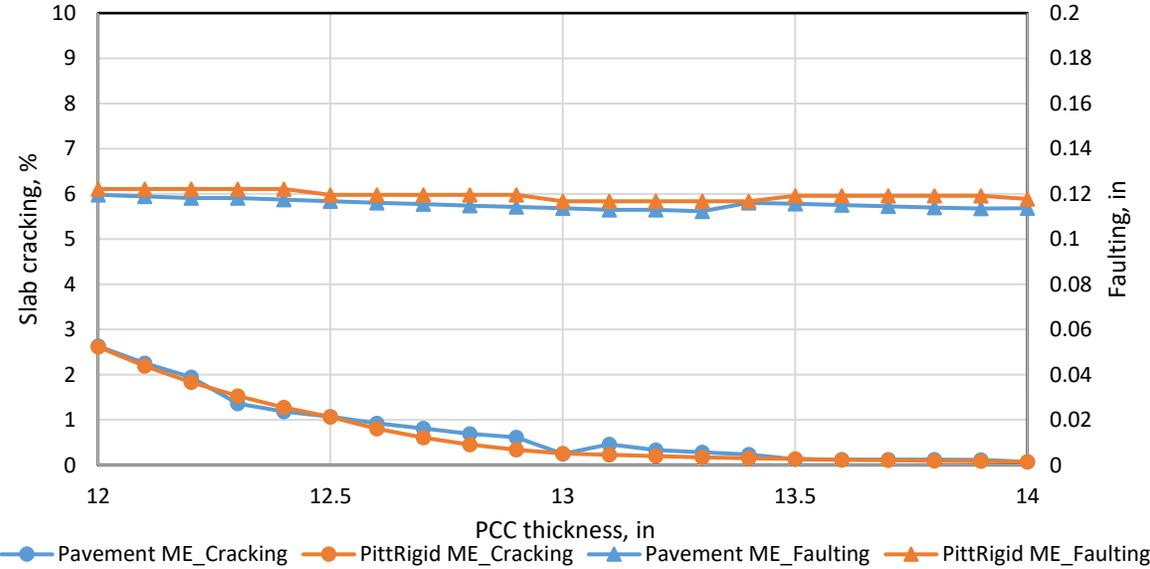
Figure 4-11. Comparing slab cracking and faulting predictions between Pavement ME and PittRigid ME at 50% reliability with respect to PCC thickness for Case 5
