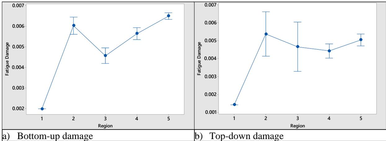
Figure A.10. Fatigue damages for 5 regions, a 9-in thick JPCP
