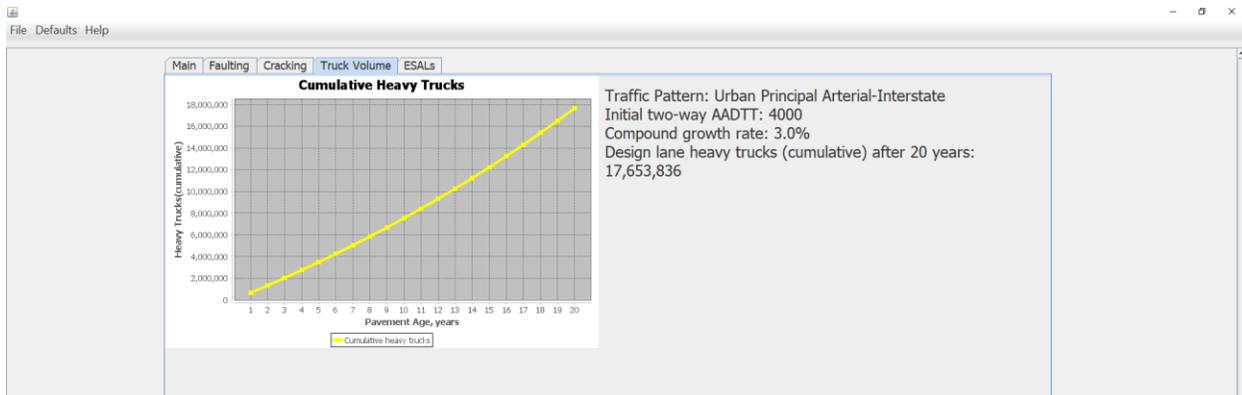
Figure 4-4. PittRigid ME screen with the results of design truck lane traffic prediction for Case 1
