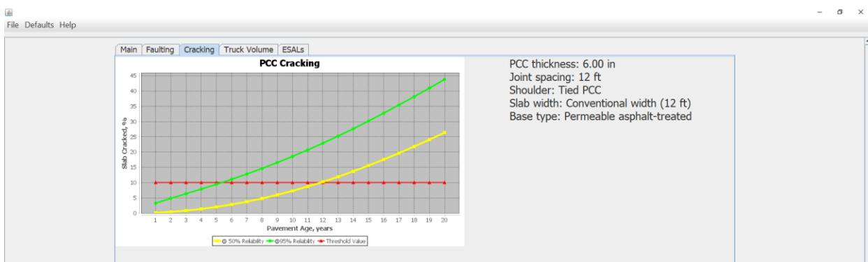
Figure 4-3. PittRigid ME screen with the results of cracking analysis for Case 1
