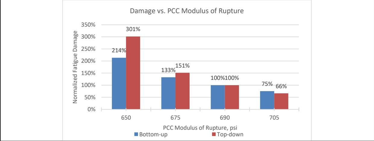
b) PCC Modulus of rupture sensitivity for fatigue damage
