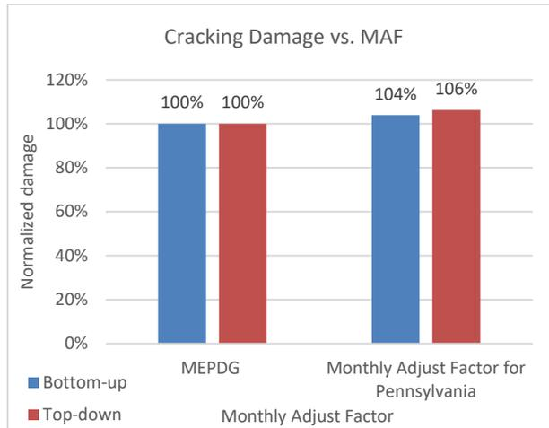
Figure A.4. Effect of truck traffic monthly adjustment factors on predicted fatigue damage
