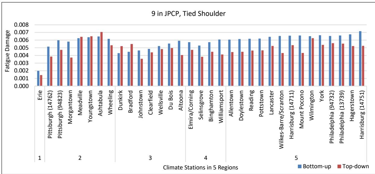
Figure A.8. Predicted fatigue damage for all climate stations, a 9-in thick JPCP
