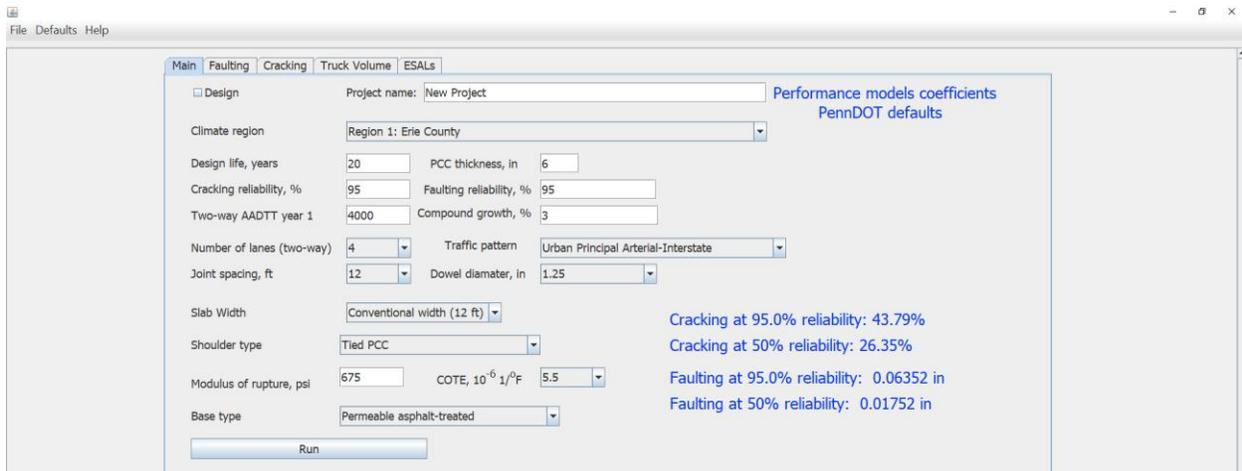
Figure 4-1. Main screen of PittRigid ME with the inputs and outputs for Case 1
