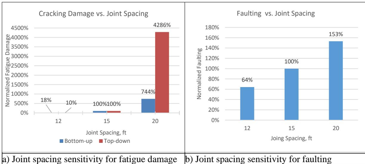
Figure A.11. Effect of joint spacing on predicted fatigue damage and joint faulting
