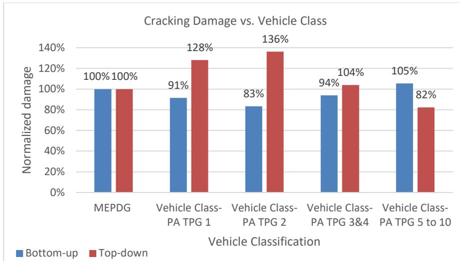
Figure A.5. Effect of the traffic pattern on predicted fatigue damage
