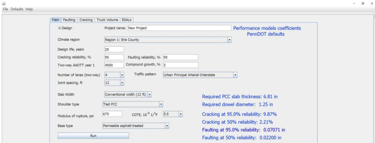
Figure 4-8. Main screen of PittRigid ME with the inputs and outputs for Case 2
