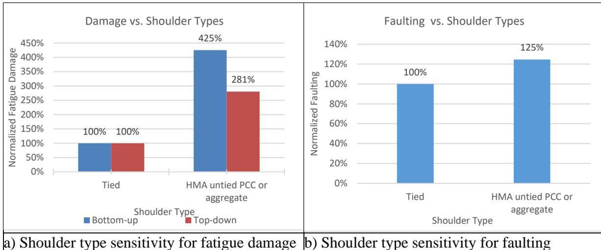
Figure A.13. Effect of should type on predicted fatigue damage and joint faulting
