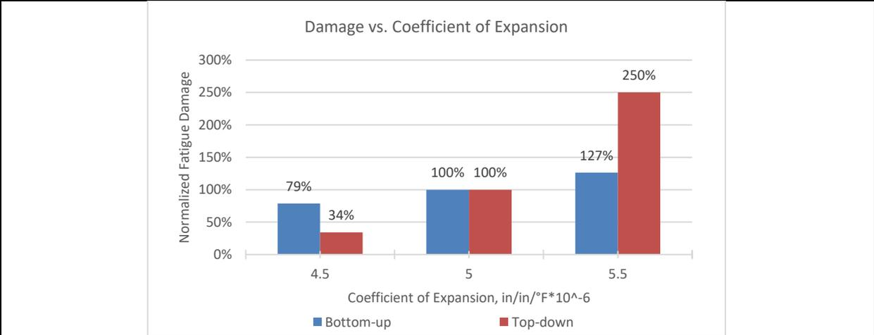
a) Coefficient of expansion sensitivity for fatigue damage
