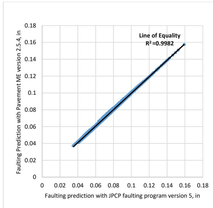
Figure 3-3. Comparisons of faulting predictions between using JPCP faulting program version 5 and Pavement ME version 2.5.4
