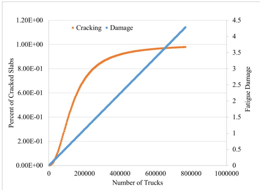
Figure A.1. Example of cracking and fatigue damage vs truck volume
