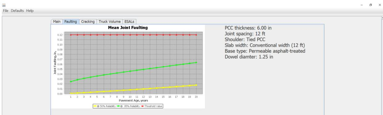
Figure 4-2. PittRigid ME screen with the results of faulting analysis for Case 1
