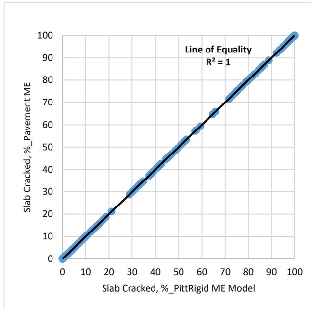
Figure 3-2. Comparison of PittRigid ME and Pavement ME transverse cracking predictions.
