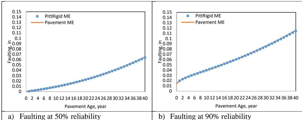
Figure 4-10. Faulting comparisons between PittRigid ME and Pavement ME for Case 3
